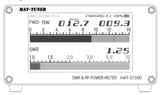
The front panel of the mAT-S1500 is a 4.3 "high-resolution color display screen.
