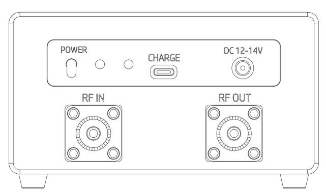
RF IN RF signal input. Connect the transmitter or amplifier.
