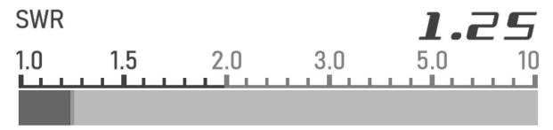
The progress bar will set different colors according to the value of SWR, which are green, yellow and monochrome. When the SWR is too high, mAT-S1500 will emit a beep to prompt the user.
